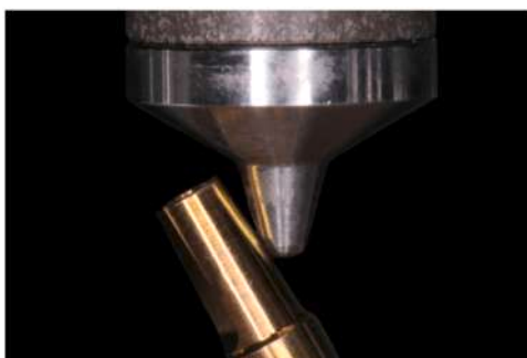
Figure 2. Dynamic mechanical load test of implant-prosthetic abutments.
